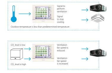
Interlock insures all system components work together, saving energy and increasing comfort.
